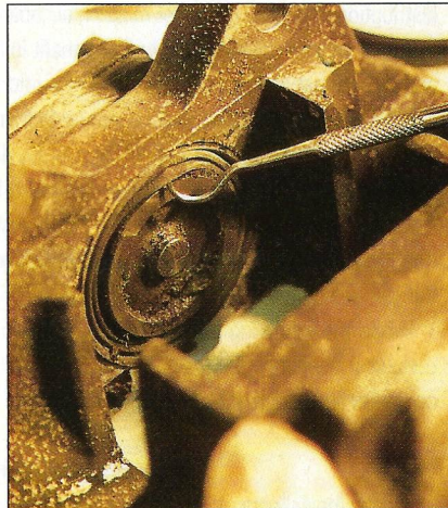
Left: Removing brake piston with high-pressure air hose. Right: Removing duct cover from brake piston.
