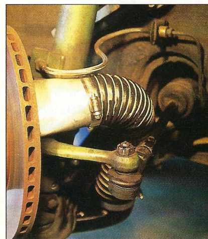
Left: Gripping difference: (top to bottom) Pagid's Orange pad for the 993 Turbo compared to the 1970 911S front pad and rear pad. Right: Cooler Brakes disc in place with hose leading to lower scoop.
