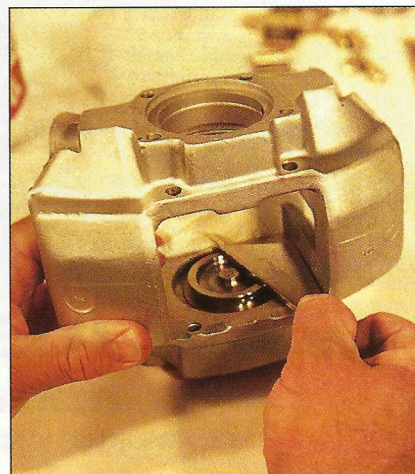
Left: Aligning the brake piston inside the S-type aluminum caliper. Right: Arrow reveals the opening in the hub where a portion of cool air is lost.
