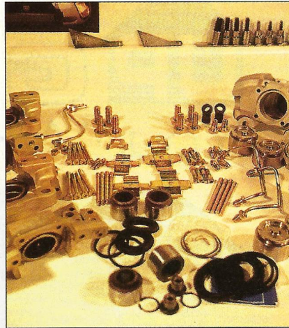
Left: Brake calipers cleaned and ready to rebuild. Right: Rear brake pistons. While the piston face (R) maybe pitted, be sure the circumference of the pistons (L) are in perfect condition.
