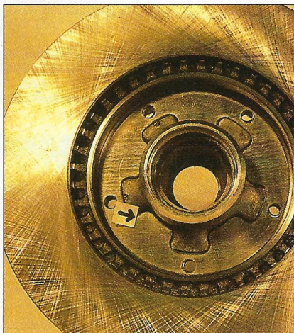
Left: With the deflection plate in place, the arrow points out how it has sealed the hub openings, where a portion of cool air can be lost. Right: The Cooler Brakes disc in place on rotor.
