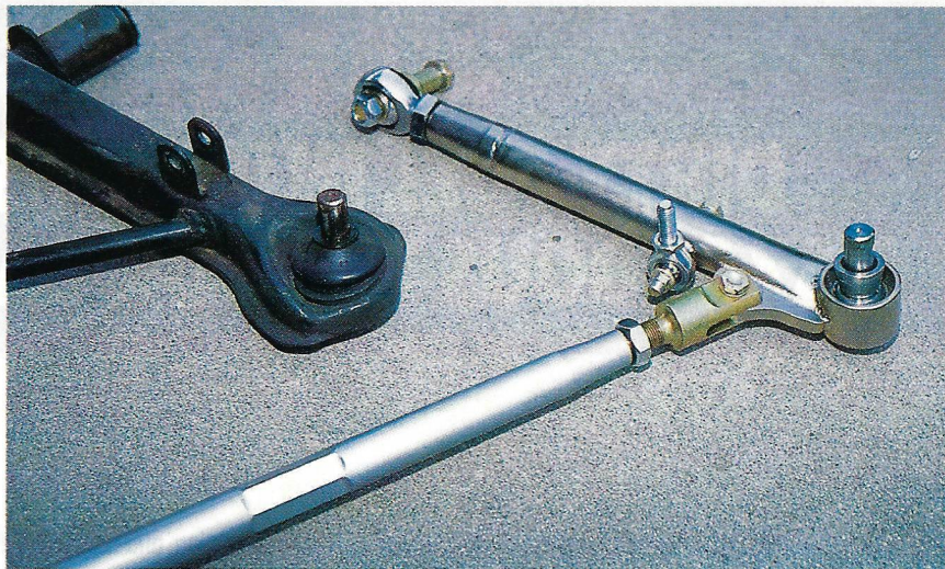
Original 911 A-arms (above) vs. E.R.P. mono-ball A-arms (below).
