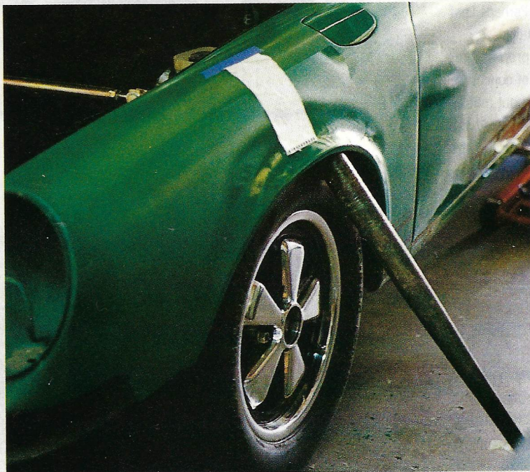
Using a wooden bat to roll the inner lip of the front fender.
