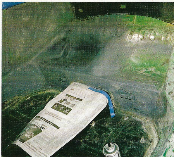
Cleaning the surface rust from the rear seat buckets.
