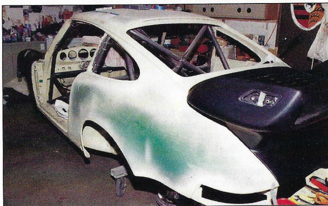
First fitting of the RSR 3.8-style bi-wing tail.
