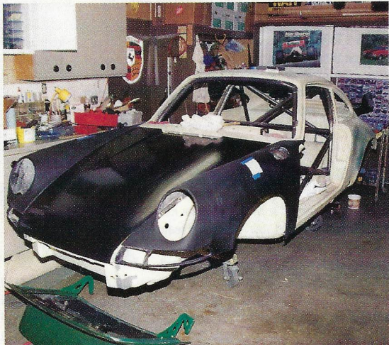
First fitting of hood and fenders.
