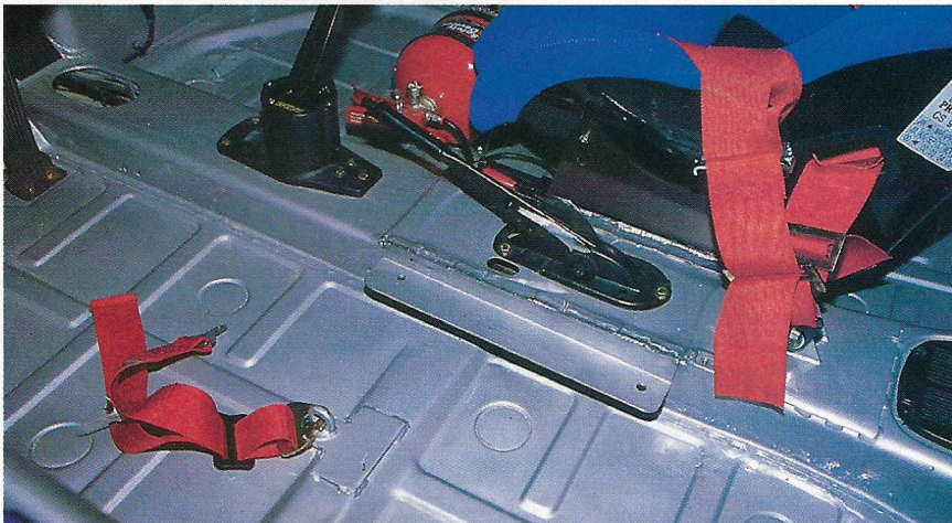
Corrected seat brackets help me fit under the car's inner roof.
