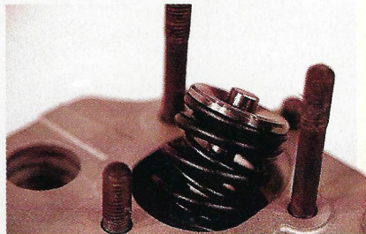
Left to right, in descending order: 1. A close up of the beveled combustion chamber. 2. S cylinder heads with titanium valve retainers and competition valve springs, Norris Performance Products and Aasco Performance. 3. Close-up of titanium valve retainer and competition valve spring. 4. The competition valve springs.
