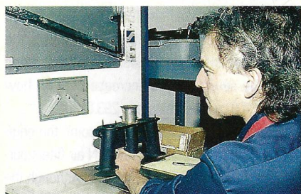
Left to right, descending: 1. Fuel injectors, new vs. old (l to r). 2. 2.7RS three-dimensional cam (right) vs. 2.2S three dimensional cam (left). 3. Refurbished 1970 911S throttle bodies. 4. Drilling 911S induction stacks for cold-start squirters. 5. 911S induction stacks with cold start squirters and fuel lines. 6. Rich Creedon works the flow bench at Performance Developments.
