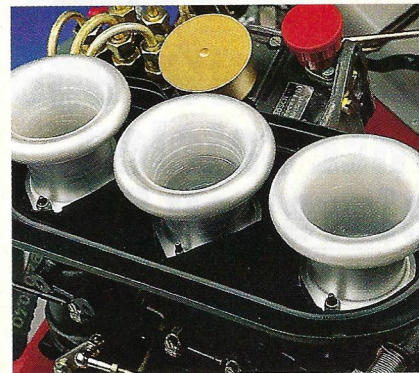
Clockwise from above: Form, function and beauty. The high-powered elegance of a Porsche 2.7-liter motor. TWM's velocity stacks top the project car's new powerplant.
