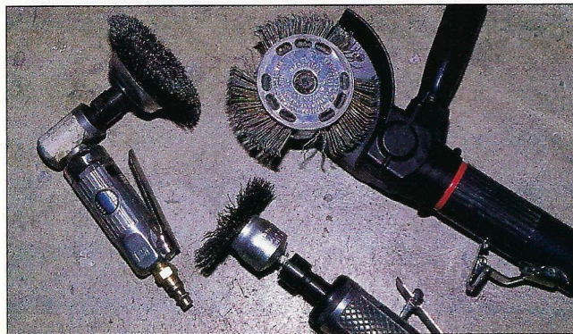
• Air tools (clockwise from top): Würth DBS 3500 pneumatic wire brush, DeVilbiss die grinder and the Campbell Hausfeld mini-angle die grinder.
