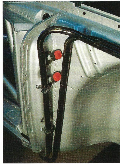
Upgraded hardlines for oil cooler.
