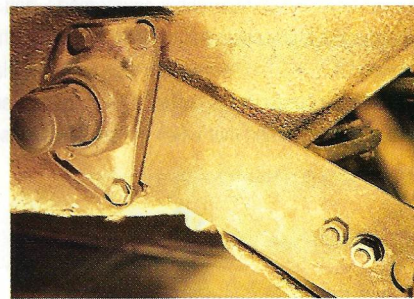
4. Late adjustable spring plate, Performance Product's adjustable Sway-A-Way spring plate. 5. Original early spring plate in place on car. 6. Late upgraded adjustable spring plate in place on car.
