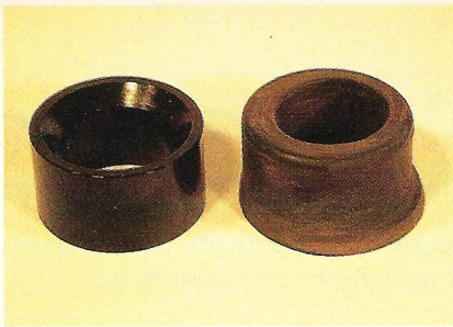
1. Tweeks polyurethane bushing and stock worn rubber bushing. 2. Tweeks polyurethane bushing and stock worn rubber bushing on stock spring plate. 3. Late adjustable spring plate, early spring plate, Performance Product's adjustable Sway-A-Way spring plate.
